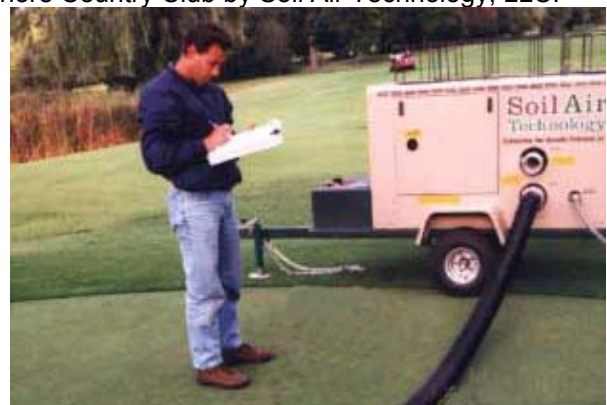
Figure 4. Sub-surface vacuum extraction equipment used at North Shore Country Club (Soil Air Technology, Middlefield, CT. www.soilair.com ). Soil CO 2 was significantly reduced after the system was run for one hour. Primarily used for dewatering greens with drainage problems, sub-surface vacuum extraction also improved infiltration rates by about two-fold. Note: this technology is covered by U. S. Patent No. 6,018,909, the use of which was licensed to North Shore Country Club by Soil Air Technology, LLC.
