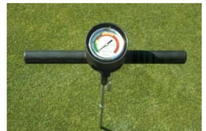
the weight of army vehicles in off road military operations. Today, this handy tool is used extensively to evaluate compaction, evaluate root growth in compacted soils, and to characterize soil physically.
