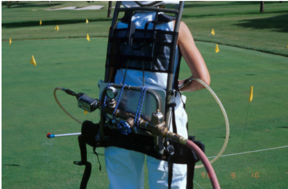
Figure 1. Set-up of backpack sprayer and flow meter used to selectively deliver irrigation to plots treated with Mach 2.
