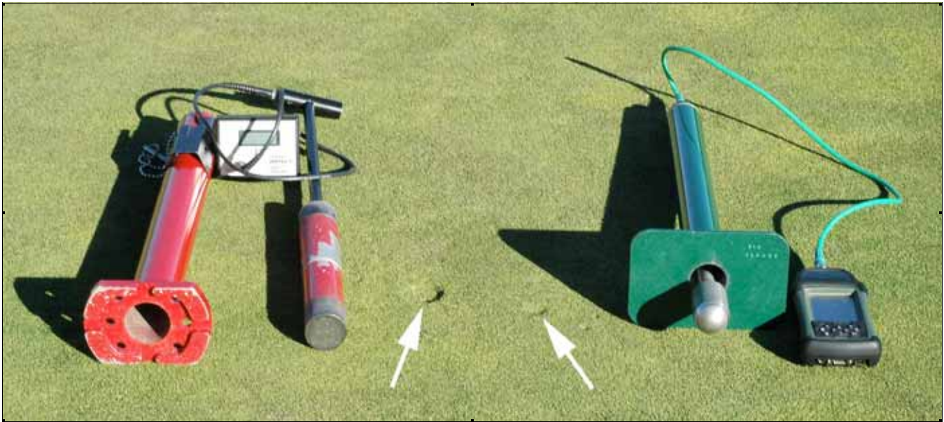
Figure 5. Comparison of turf damage produced by Clegg Impact meter (left) vs. the USGA TruFirm (right). January 12, 2009, Victoria Golf Club.
